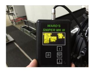
10.Offset setup. Measure from the front face plate of the MK 3 to the film plane of the camera. For example: the offset measurement is 14 inches, on the Display press the menu button, scroll up or down until the cursor is beside the offset in the menu. Press enter and the cursor moves over to the increments. Either Metric or ANSI is chosen at this point. Select which
