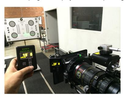
Power button is pushed on Display. This is the pairing, once the Logo disappears and measurements start, the unit is paired and doesn't need to be repeated again. (This pairing happens first at our facility and is a double check only for new purchases.) If a second display (sold separately) is
