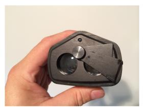
Iris up to 80% coverage of one of the lenses, regardless of the Sniper position is right side up or upside down. We say this because some instances AC's like to mount the pan and tilt bracket differently, the coverage is the same for the Smoke Iris.
